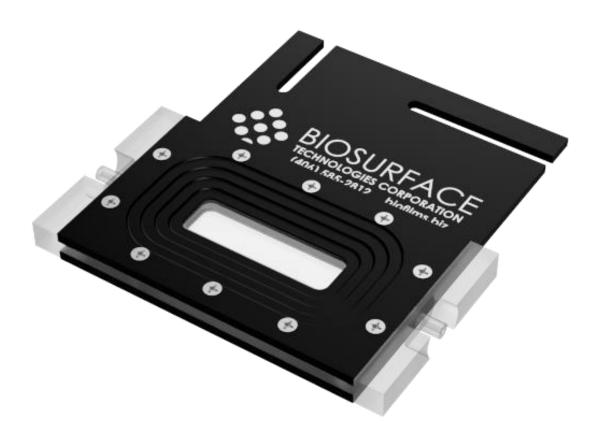
The model FC 81 / 85 flow cell consists of a polycarbonate or anodized aluminum flow channel. A glass viewing port allows transmission microscopy of biofilm growth in the flow channel.
