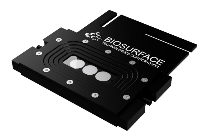
The model FC 71 / 75 flow cell consists of a polycarbonate or anodized aluminum flow channel. A glass viewing port allows reflected light microscopy of biofilm growth on coupons and in the flow channel.
