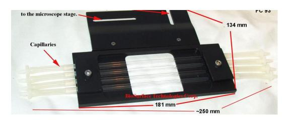
FC 93 Capillary Flow Cell (3-mm ID square glass capillary flow cell, 4 channel) \$550.00 includes: standard platform-stage microscope mount, 4 glass capillary flow channels
