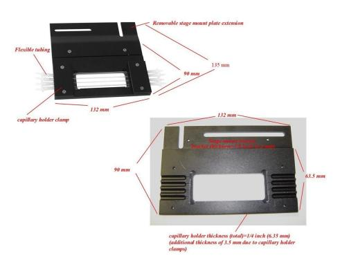
FC 91 Capillary Flow Cell (1-mm ID square glass capillary flow cell, 4 channel) \$480.00 includes: standard platform-stage microscope mount, 4 glass capillary flow channels
