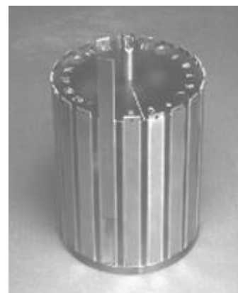
Figure 12 – Inner Cylinder with 20 Slide Coupons
