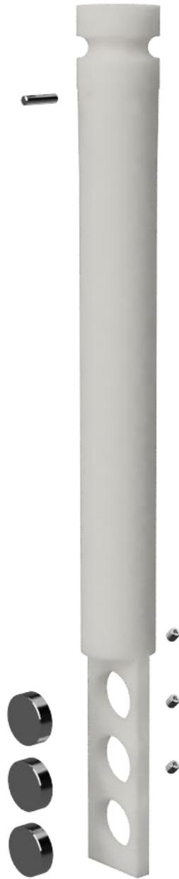
**Figure 3. Expanded schematic of coupon rod and coupons.**
