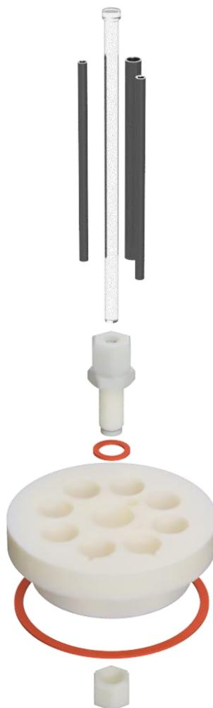
**Figure 2. Expanded schematic of reactor top.**
