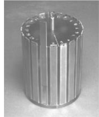
Figure 12 – Inner Cylinder with 20 Slide Coupons
