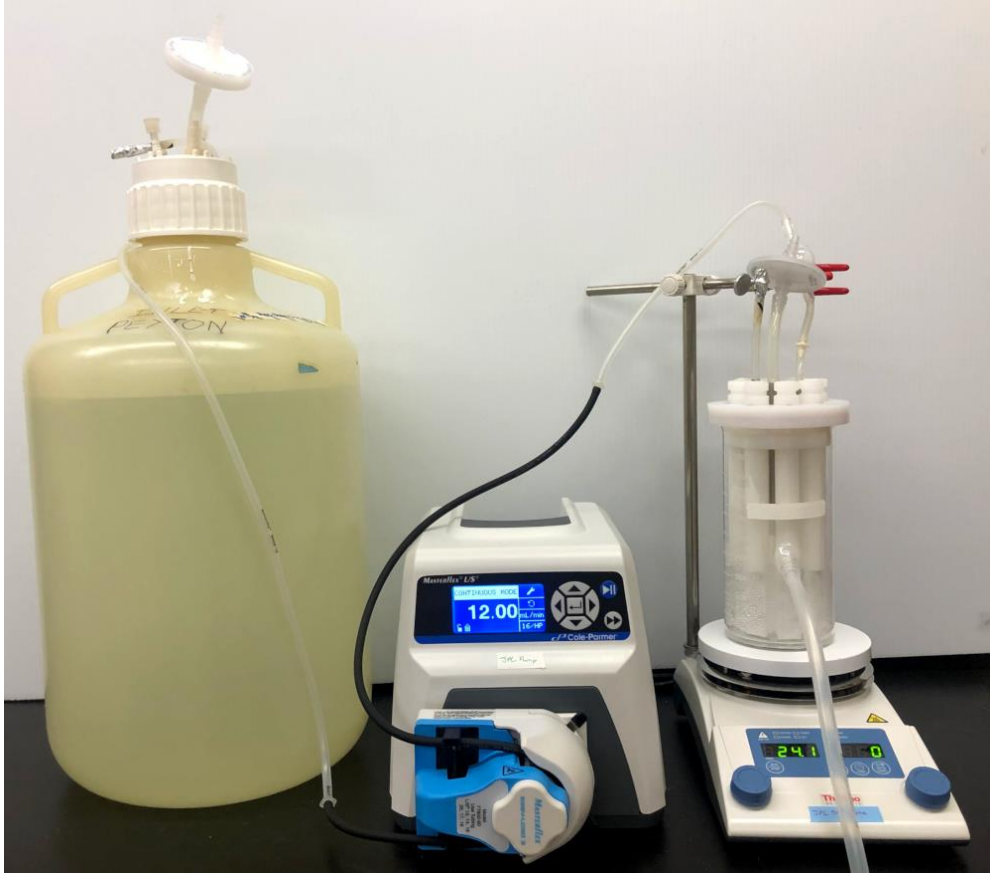
Figure 2b. Picture of an assembled reactor system (M. Mettler, CBE, 2020).
