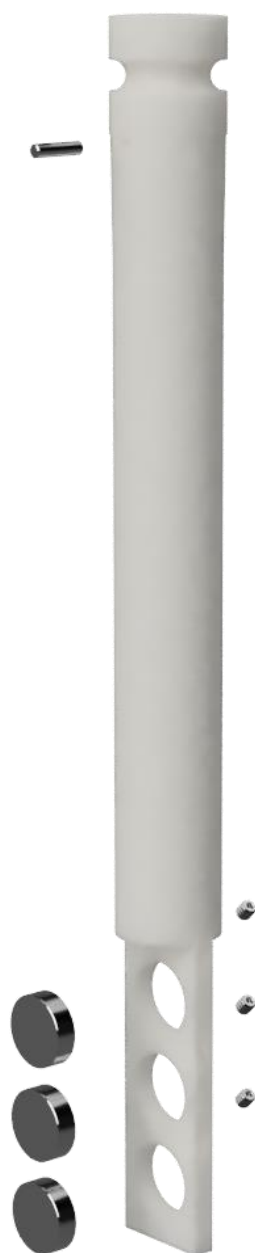
Figure 3. Expanded schematic of coupon rod and coupons.
