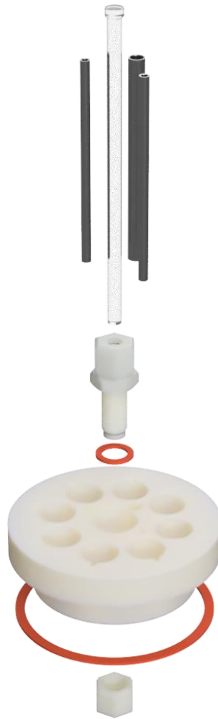
Figure 2. Expanded schematic of reactor top.
