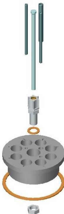
**Figure 2. Expanded schematic of reactor top** (Norris, 2003).
