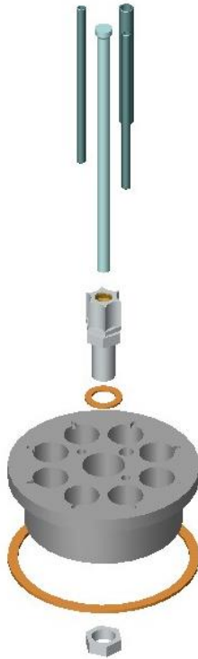
Figure 2. Expanded schematic of reactor top (Norris, 2003).
